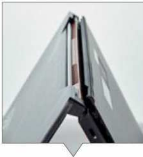
The bottom panel opens up when the lid is open.
