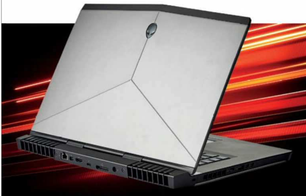
The thermal system is housed toward the rear of the chassis.
