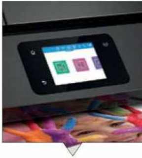
The printer's 2.65-inch capacitive touchscreen isn't very big, but it is responsive.
