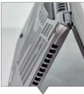
Exhaust vents at the left mean that you won't be bothered by hot air if you're using a mouse.
