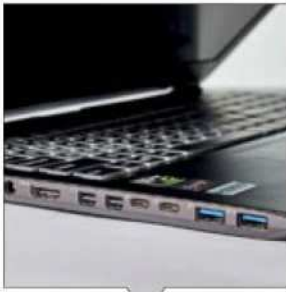
The laptop comes with two USB 3.1 (Gen 2) Type-C ports.
