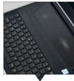
The see-through panel above the keyboard doubles as a trackpad as well.
